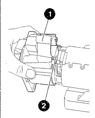
Assembling commutator end shield
